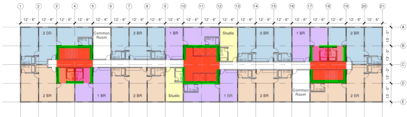
Figure 5: Typical Building Floor Plan (Core areas are highlighted in red, core walls are highlighted in green)
